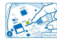
Within 2 minutes, press the WPS button inside the iAquaLink 2.0. The two devices will exchange a passcode and establish communication.
