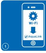
After clearing the Wi-Fi settings and with the Wired/Wi-Fi switch set to Wi-Fi, use a smartphone or Wi-Fi enabled device to go to Wi-Fi settings. Connect to the network labeled iAquaLink.
